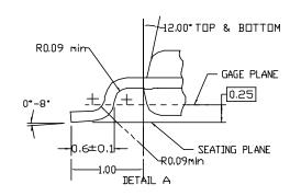
Figure 3. 14-Lead Thin Shrink Small Outline Package (TSSOP), JEDEC MO-153, 4.4mm Wide Package MTC14
